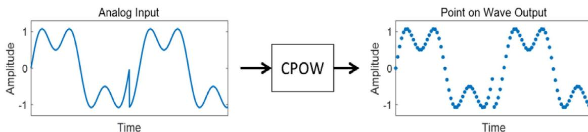
Figure 5: Conversion of an analog input to a point on wave output.<sup>1</sup>
