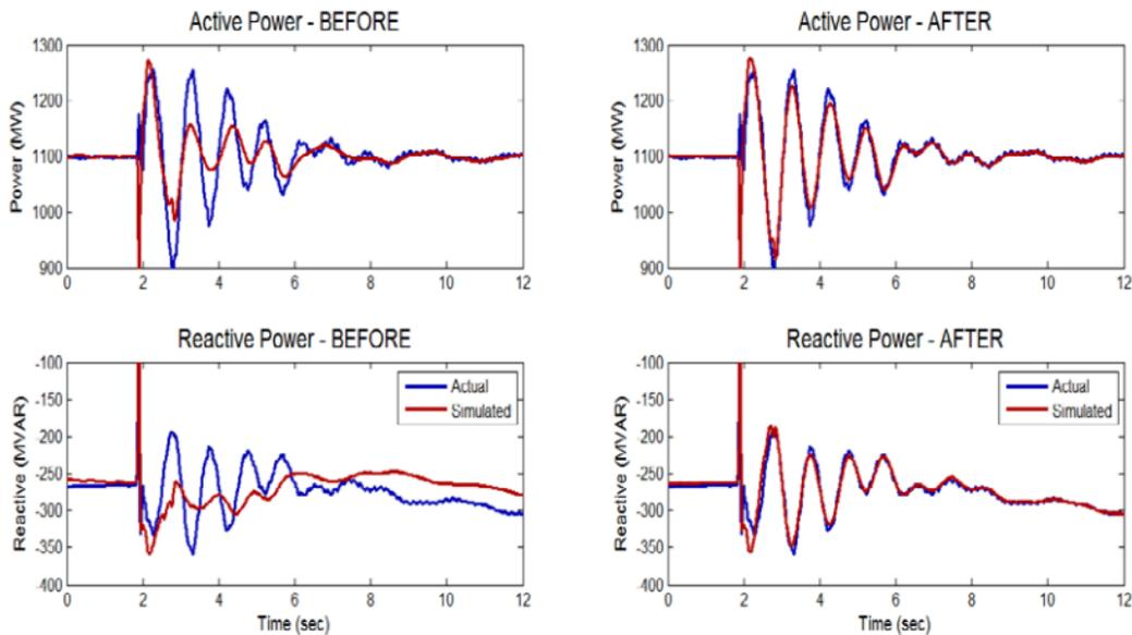
Figure 11. Power plant model validation before and after calibration (source: BPA)
