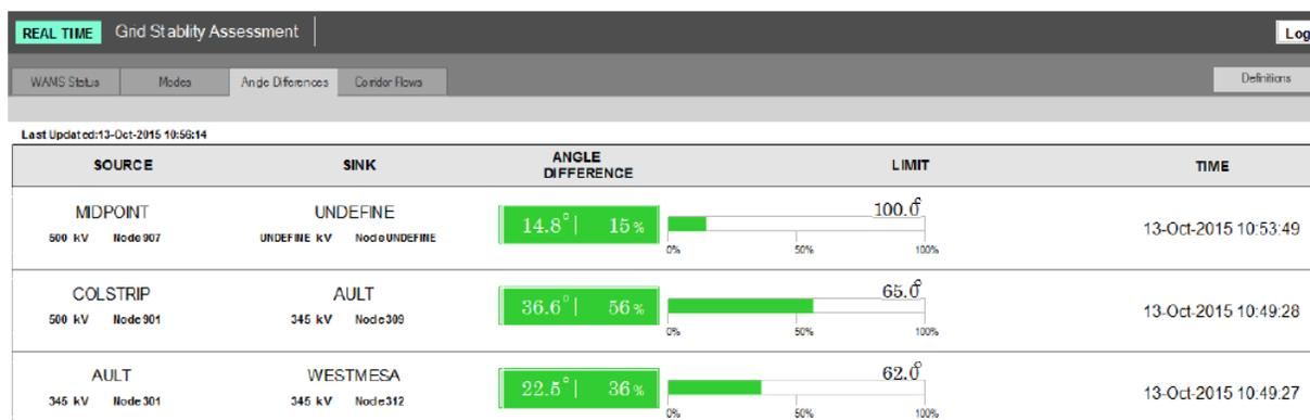
Figure 9. Synchrophasor-based angle alarming (source: Peak Reliability)
