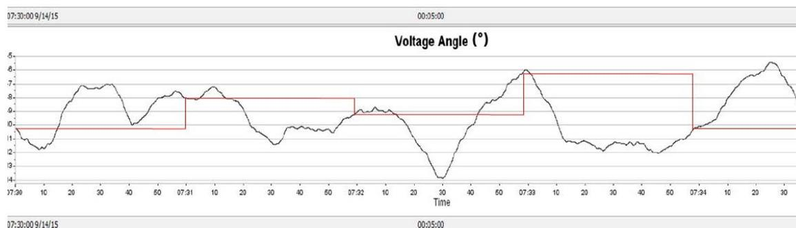
Figure 8. Phase angle from PMU (black) vs. state estimator (red) (source: Peak Reliability)
