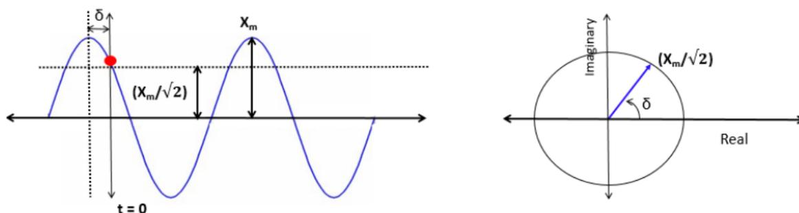
Figure 1: Illustration of a phasor estimate from a continuous waveform
