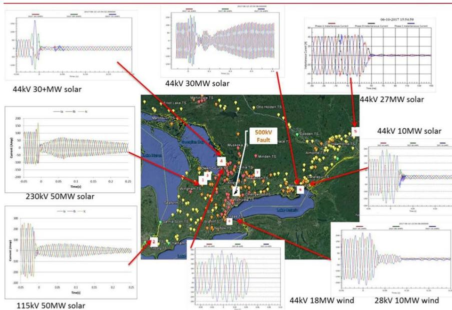
Figure 13. HydroOne renewable monitoring – system wide event (Source: Chester Li<sup>1</sup>)
