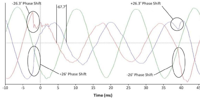
Figure 12. Phase jump at fault location during Blue Cut Fire Disturbance (Source: NERC)
