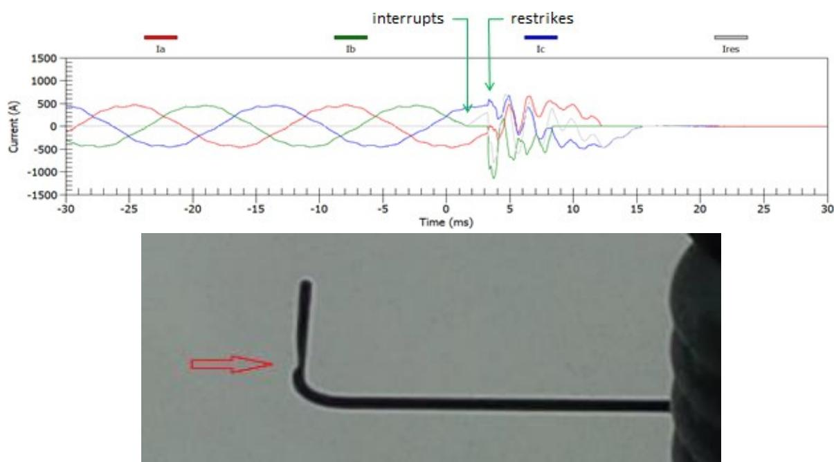
Figure 16. Waveform with restrike of a capacitor bank (upper) and Pitted arcing horn of a capacitor bank (lower)<sup>2</sup>
