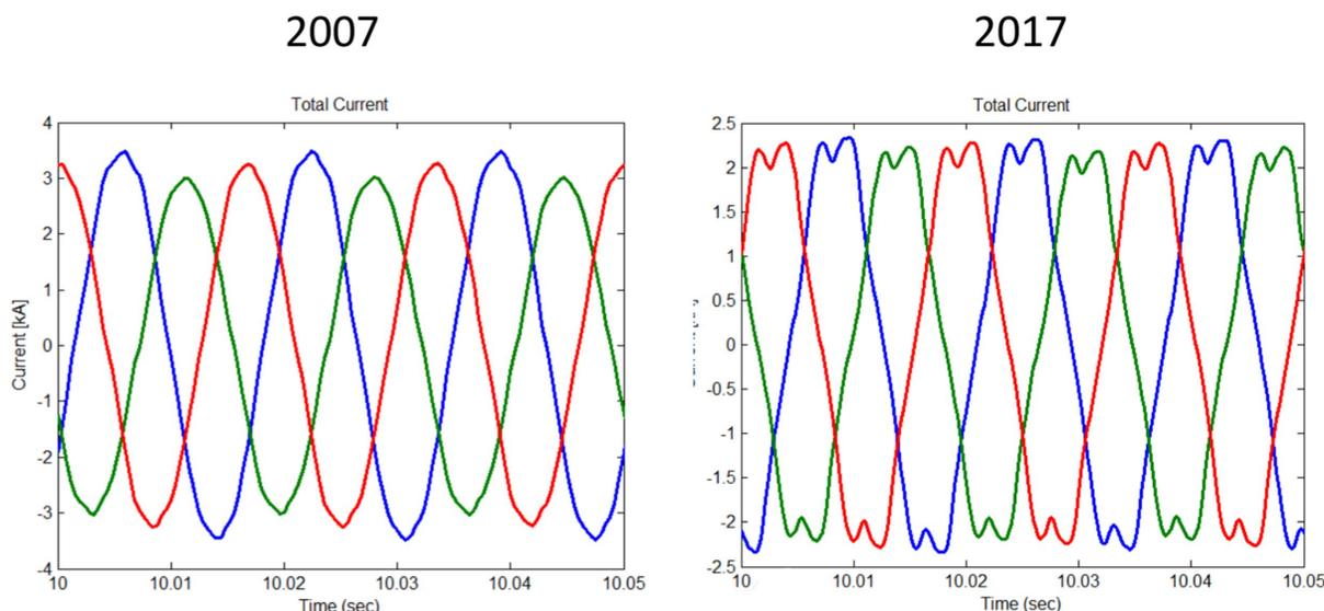
Figure 15. Commercial building POW measurements (Source: BPA<sup>1</sup>)
