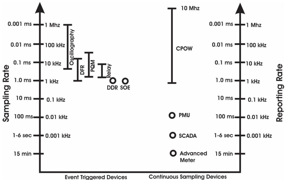
Figure 18: Grid monitoring devices by resolution and data continuity<sup>1</sup>.
