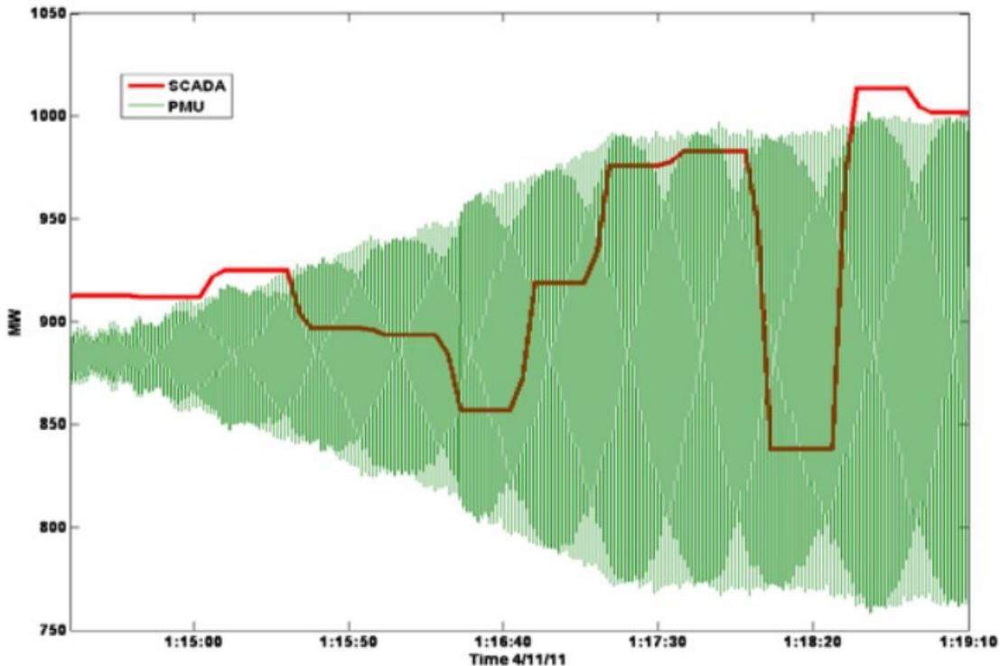
Figure 2: Synchrophasor data provides a much more detailed representation of an oscillation than SCADA data at its much lower time resolution (Source: Dominion)
