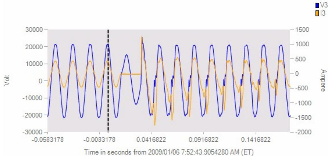
Figure 17. Zero current waveform data during transformer load tap changer failure<sup>1</sup>
