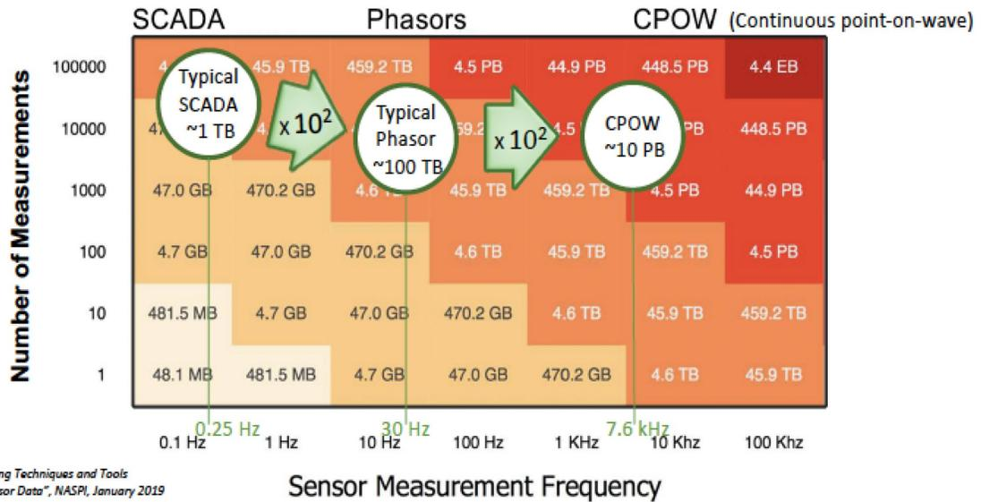
Figure 19: Annual data storage requirements as they increase for SCADA, synchrophasors, and CPOW (Source: NASPI<sup>1</sup>)
