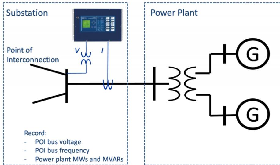
Figure 10. Power plant model validation concept (source: BPA)
