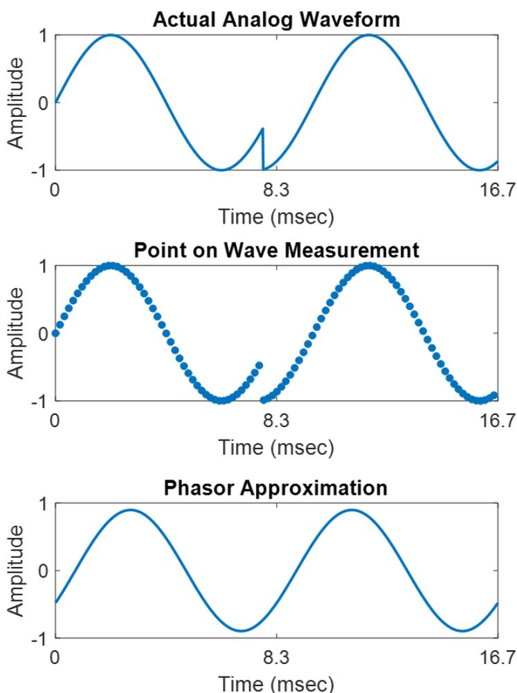
Figure 6. An analog waveform (top), its representation as POW measurements (middle), and its reconstruction from a phasor estimate (bottom).
