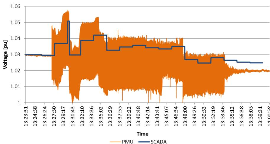
Figure 7. Forced oscillation observed with SCADA and PMU data (source: ATC)
