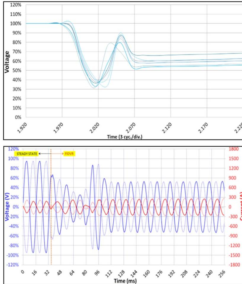
Figure 14. FIDVR event captured in voltage magnitude measurements (top) and POW measurements (bottom) (Source: SCE<sup>1</sup>)
