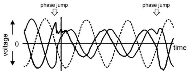
Figure 4: NERC graph based on DFR data, showing phase jumps that were interpreted as a major drop in frequency. Solid lines are the actual data, while the dashed line is a sinusoid shown for reference. (Source: NERC<sup>1</sup>)
