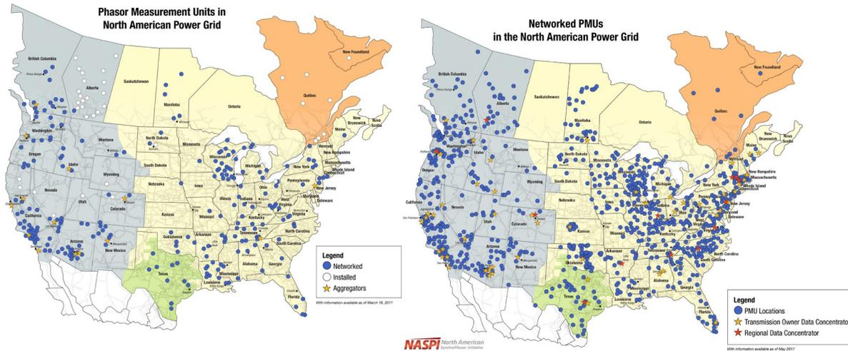
Figure 3. North American Power Grid PMU map 2011 vs. 2017 (Source: NASPI<sup>1</sup>)
