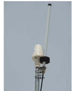
Figure 10 – Interference from a close RF source can jam GPS reception
