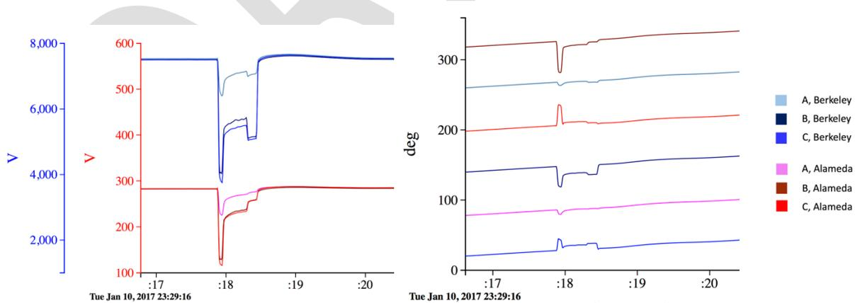
Figure 2: Voltage magnitudes and angles during a disturbance event at two locations separated by the transmission grid and multiple delta-wye transformers (UC Berkeley, LBNL).
