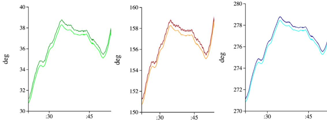
Figure 1: ABC phase alignment between two locations on a distribution circuit as seen by micro-PMUs on the Berkeley Tree Database (BTrDB) plotter (UC Berkeley, LBNL).
