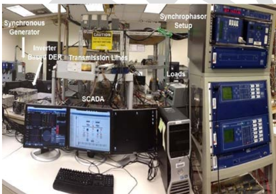
Figure 1: Microgrid involves a synchronous generation unit, an inverter based DER and local loads. Connection to utility grid enables both is-grid-connected and islanded operation. Operational voltage is 208 V RMS line-to-line as utility voltage level . (Smart Grid Test Bed at Florida International University)
