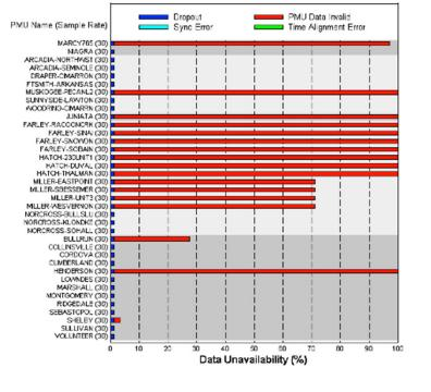
Out of 111 networked eastern PMUs, only 29% were delivering >95% data on 12/9/11 – most poor-performing PMUs due to communications problems.
