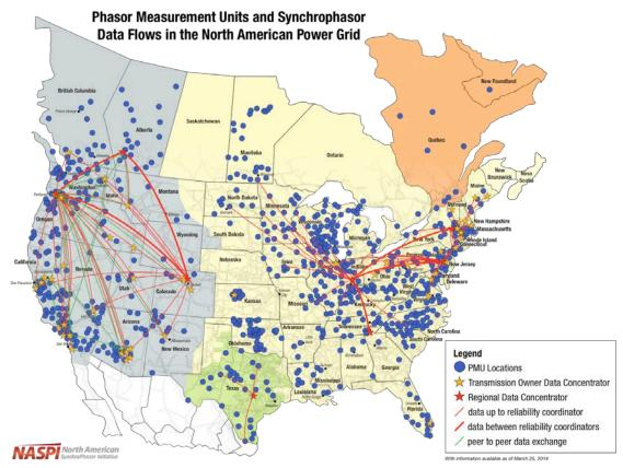
In 2009 there was little data-sharing of synchrophasor data between grid operators. Today there is extensive sharing of synchrophasor data thanks to the U.S. Department of Energy Smart Grid Investment Grant (SGIG)-assisted synchrophasor technology build-out.
