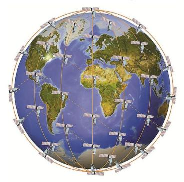
**Iridium Nominal Constellation** 66 Satellites in 6 Orbital Planes **11 Satellites in each Plane** 781 km Altitude, Polar orbits (86.4 degrees) Orbital speed 27,000 km/hr (17k mph) Orbital period 100 minutes (14x/day) Different satellite in each plane every 9 min
