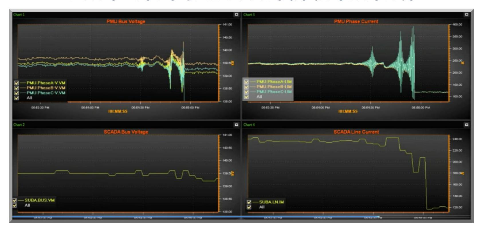
Comparison of full stream sub-second PMU measurements and SCADA data taken during testing of new generator control settings that caused unit output to swing rapidly and result in voltage oscillations on the 138 kV system.
