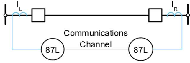
Line differential relays (device 87L) compare the local line current ( $I_L$ ) and remote line current ( $I_R$ ) to determine whether a line fault (i.e., short circuit) has occurred.
