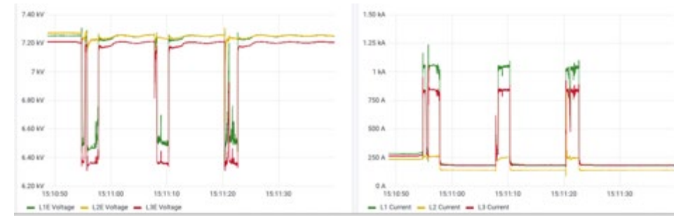
Line reclosers open/close (vegetation)
