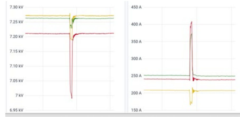
Line recloser open (wire down)
