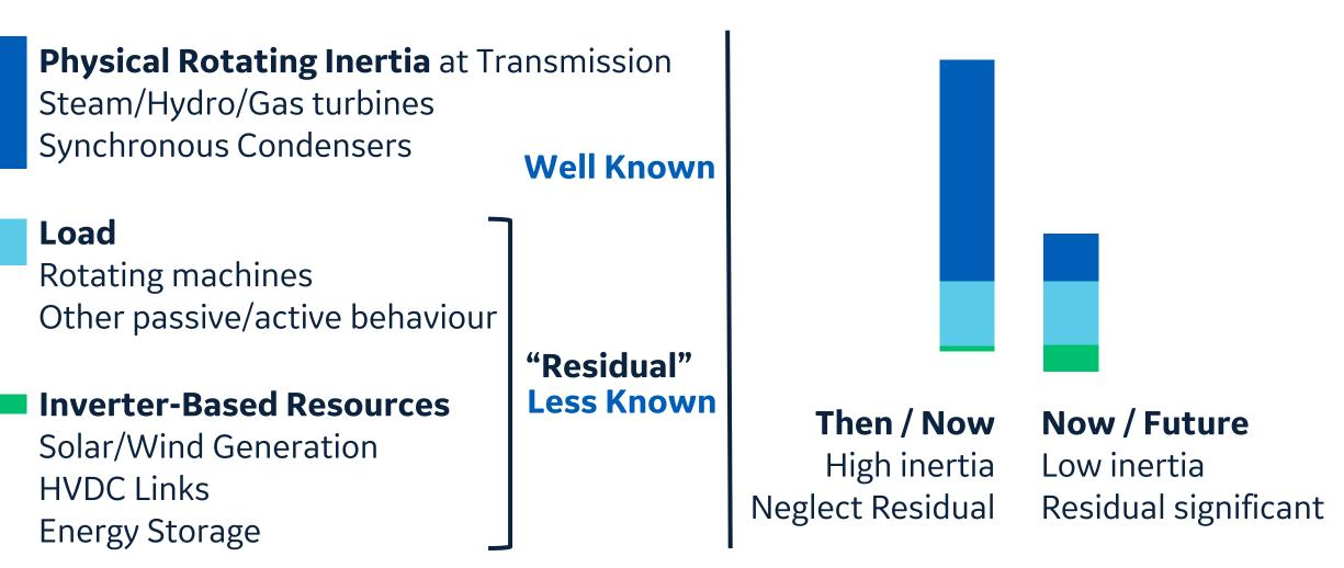
Measurement & Forecasting of Effective Inertia is becoming critical to grid operation
