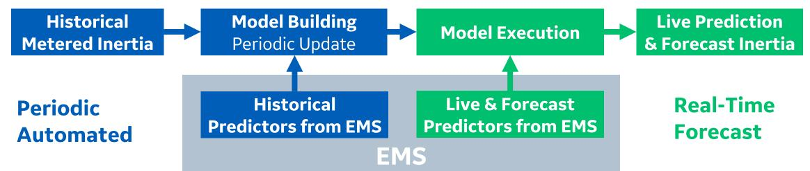
Machine Learning model links inertia to predictor variables, on a per-area basis: E.g. Demand, Synchronous Inertia, Wind, Solar
