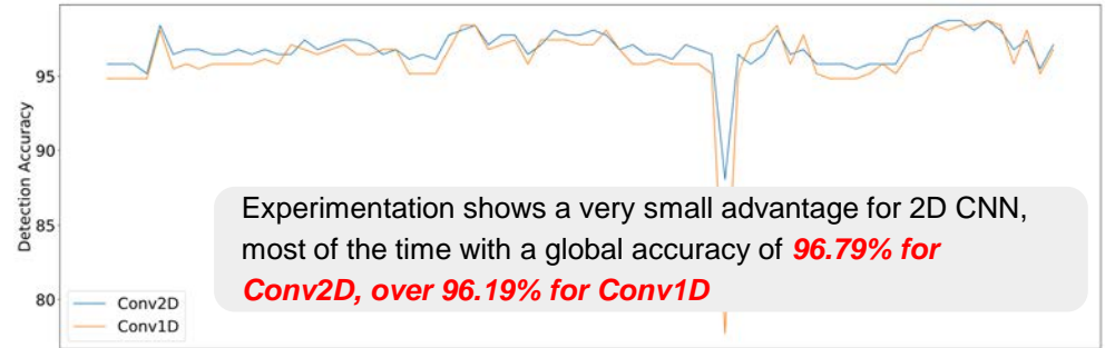
Each point on the x-axis is a different terminal (transmission line substation end). 2 minutes of normal events then 2 minutes of oscillation events)
