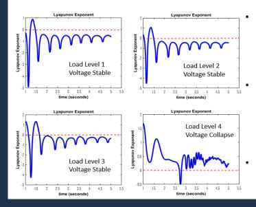
LE data for 4 cases with the same operating conditions but different voltage sensitive area loads over a window of 5 seconds for a 500 kV Line Trip Event
