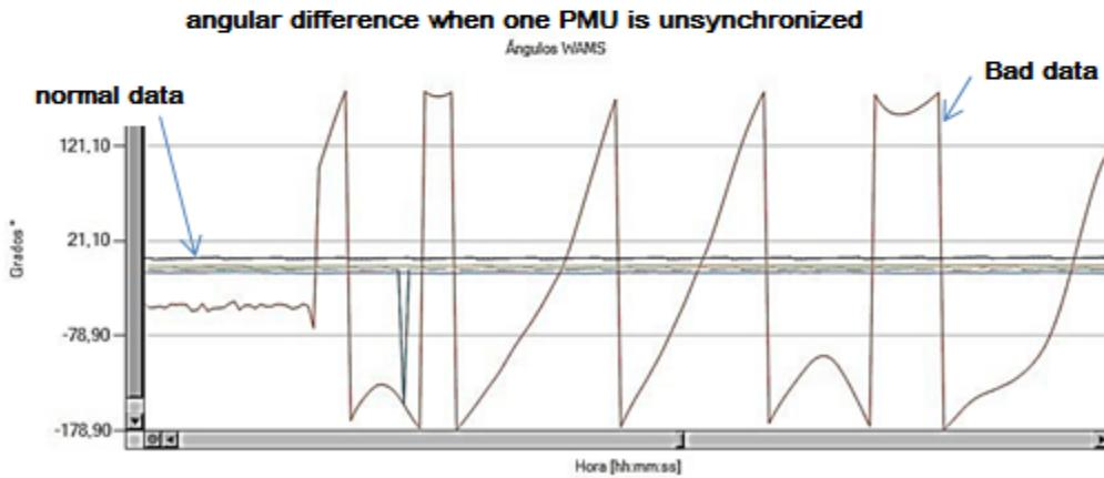
It is obtained when one PMU is unsynchronized.
