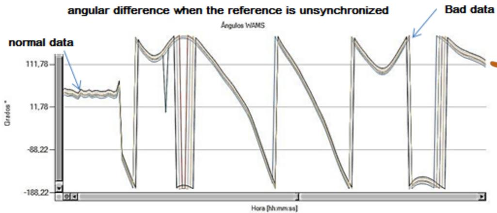
It is obtained when the reference is unsynchronized.
