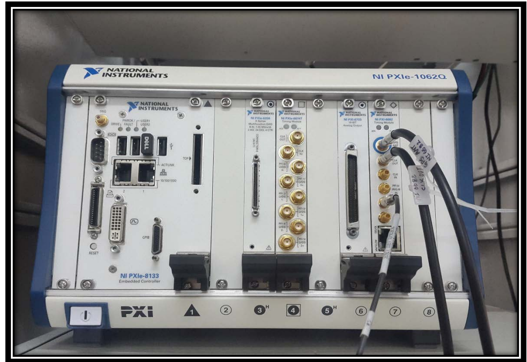
NI Controller with IO & Communication Cards
