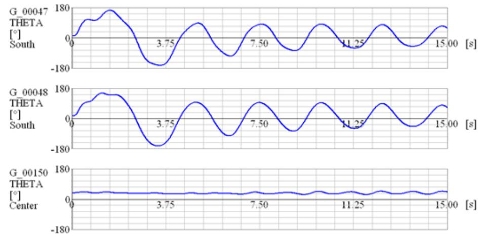
Swings of Generator pole angle with high amplitude
