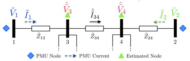
• Bus 3 is redundant: its voltage phasor can be computed independently from the PMU data at Buses 1 and 2.
