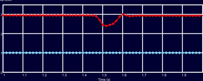
Remote bus side phase B voltage synchrophasor Synchrophasor data check
