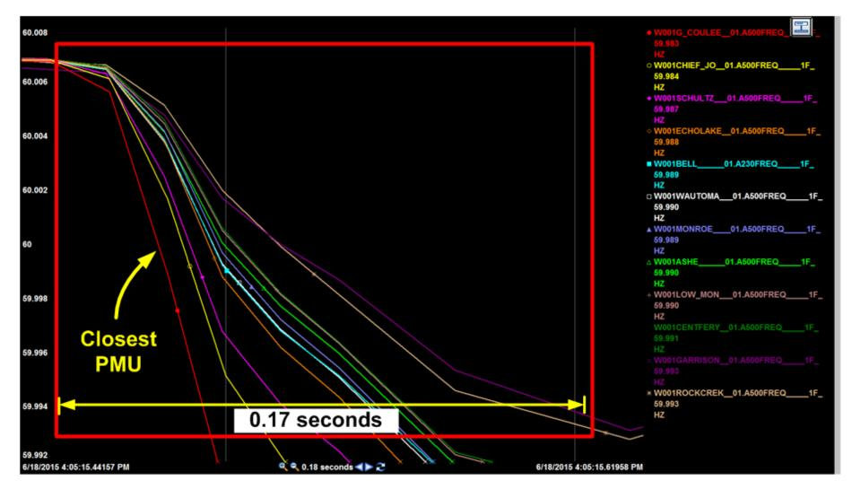
Have found that best results are obtained when calculating the freq rate-of-change (slope) after a relatively small freq drop.
