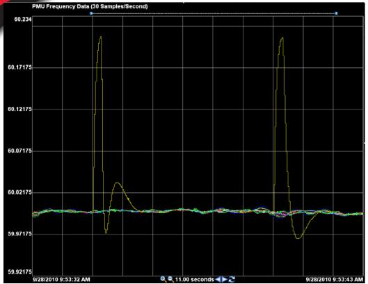
We noticed significant frequency excursions from several of our installed PMUs that were found to be due to a firmware issue in our PMU devices. These occur when GPS clock signal is lost.
