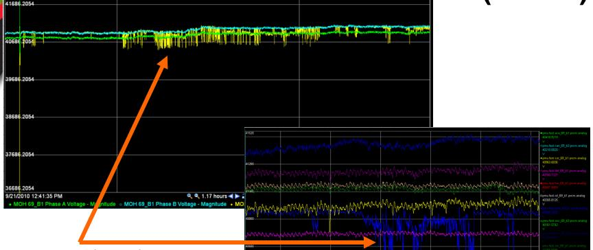
Voltage traces showed significant noise following a 69 Kv line fault. This noise was traced to a switch that was found to be arcing at a tap pole at a nearby station.
