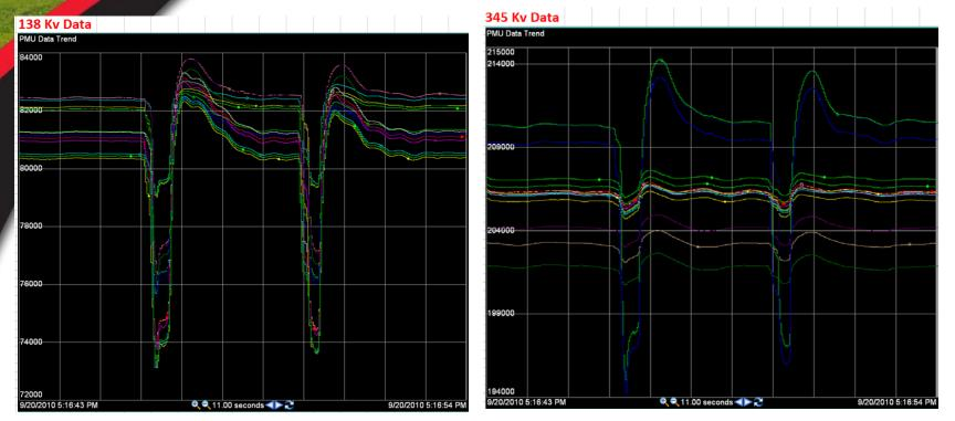
A recent three phase 69 Kv fault occurred in south central Wisconsin. We were able to observe the impact at stations scattered across our footprint. The 138 kv and 345 kv voltage traces are shown above.
