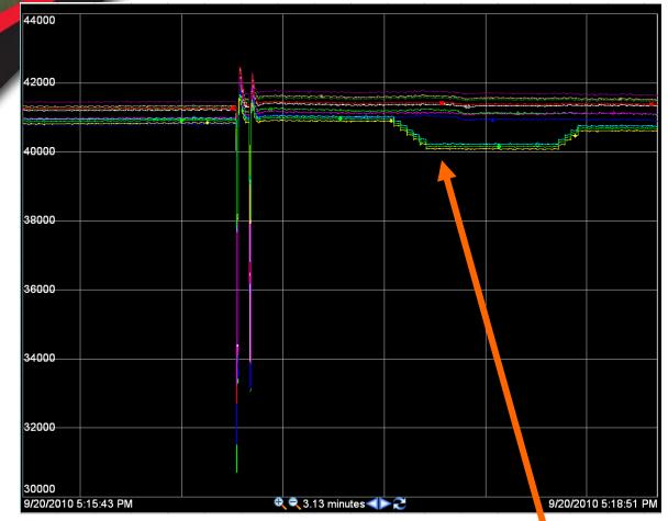
A significant fault on the 69 Kv system caused an incorrect LTC operation at a nearby bus a short time after the event. Having the time synched data allowed easy correlation of events whereas this would have been undetected prior to PMU data being available.
