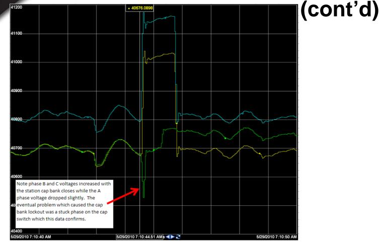
Voltage traces from a nearby station could have been used to confirm a stuck phase on a cap bank switch that was closed in and eventually tripped back out.
