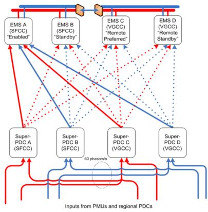
Multi-host Redundancy (ISD Link)
