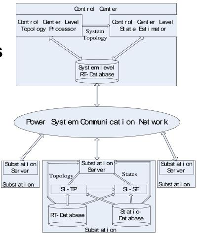
SL-TP: Substation Level Topology Processor
