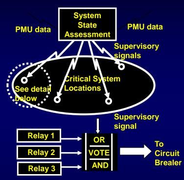
Adjustment of Dependability-Security balance under stressed system conditions.
