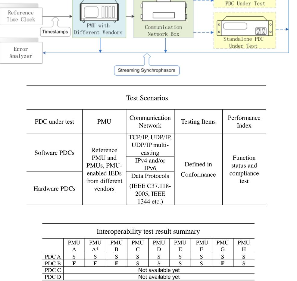
\* PMU A-1 is an upgraded firmware of PMU A
