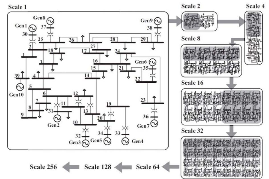
Fig. 2. Construction of test systems for transient stability simulations. The Scale 1 system shows the one-line diagram of the IEEE's New England Test System
