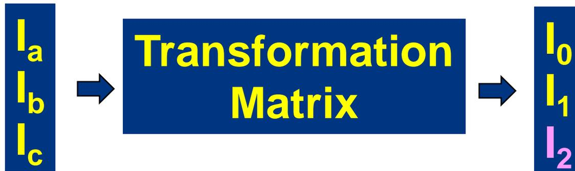
$I_2$  is the negative sequence current, which is most harmful to generators.
