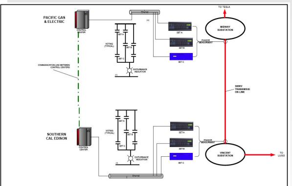
Dependability (Reliability): High probability that relays will operate for an actual fault. Security: Low probability that relays will operate when there isn't an actual fault.
