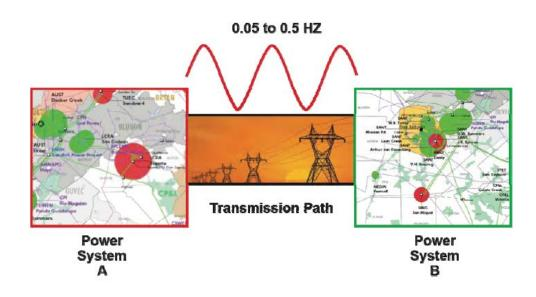
Early warning of poorly damped lines allows operators to react before an event triggers an inter-area oscillation
