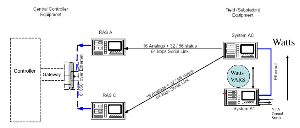
Use of high speed serial links (Up to T1 level) and Interface with GOOSE Messaging
