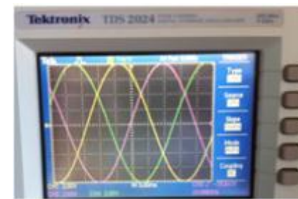
Monitoring Output Measurement (3-Phase signals)
