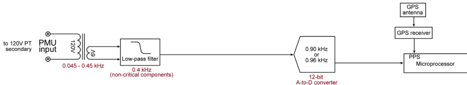
Traditional PMU, optimized for transmission system Partial schematic, showing analog path for typical \pm 1^\circ angle resolution
