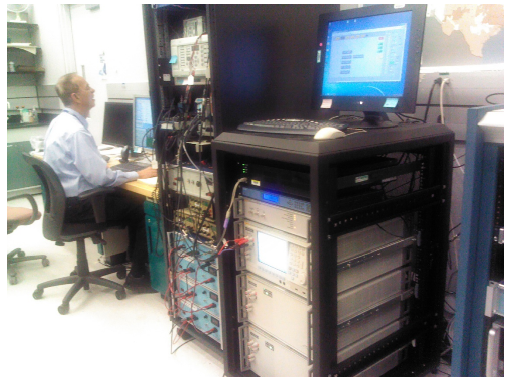
Left: Jerry Stenbakken Bottom: NIST's first PMU dynamic test system, Right: Fluke Calibration's commercially available, fully automated PMU calibration system.
